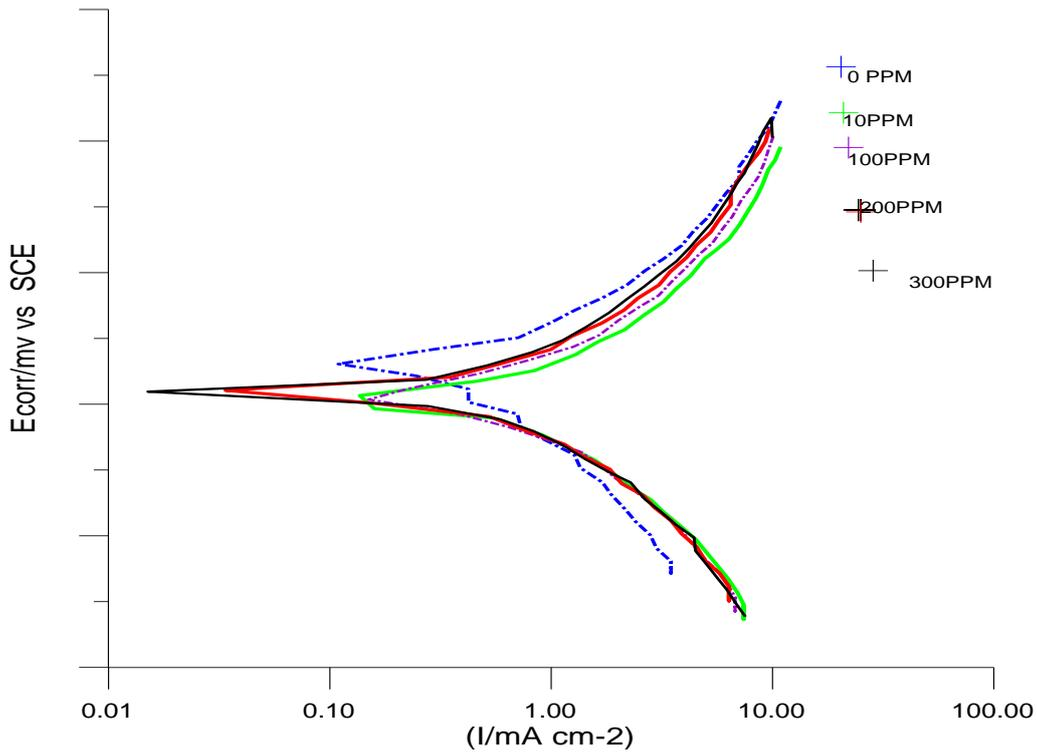
**Fig 1: Potentiodynamic Polarization curve of carbon steel with different concentrations of voltaren drug in 0.2N HCl at 25 °C**
